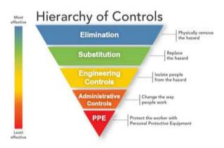
Engineering controls aim to reduce the spread of pathogens and reduce the contamination of surfaces and inanimate objects. This would include isolating a confirmed/suspect COVID-19 patient by placing them in a private negative pressure room or installing barriers to isolate staff from the risk (i.e. screening desks).
